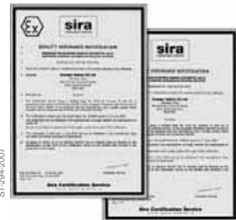
Approvals. ATEX performance approved systems require a supporting Quality Assurance Certificate from a Notified Body.
