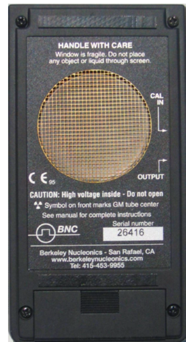
The back panel of the palmRAD 907 (shown above) features the 2-inch pancake GM detector.
