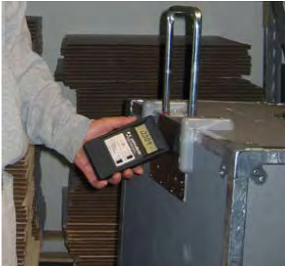
palmRAD 907 (shown left) being used to locate radiation and measure in uR.
